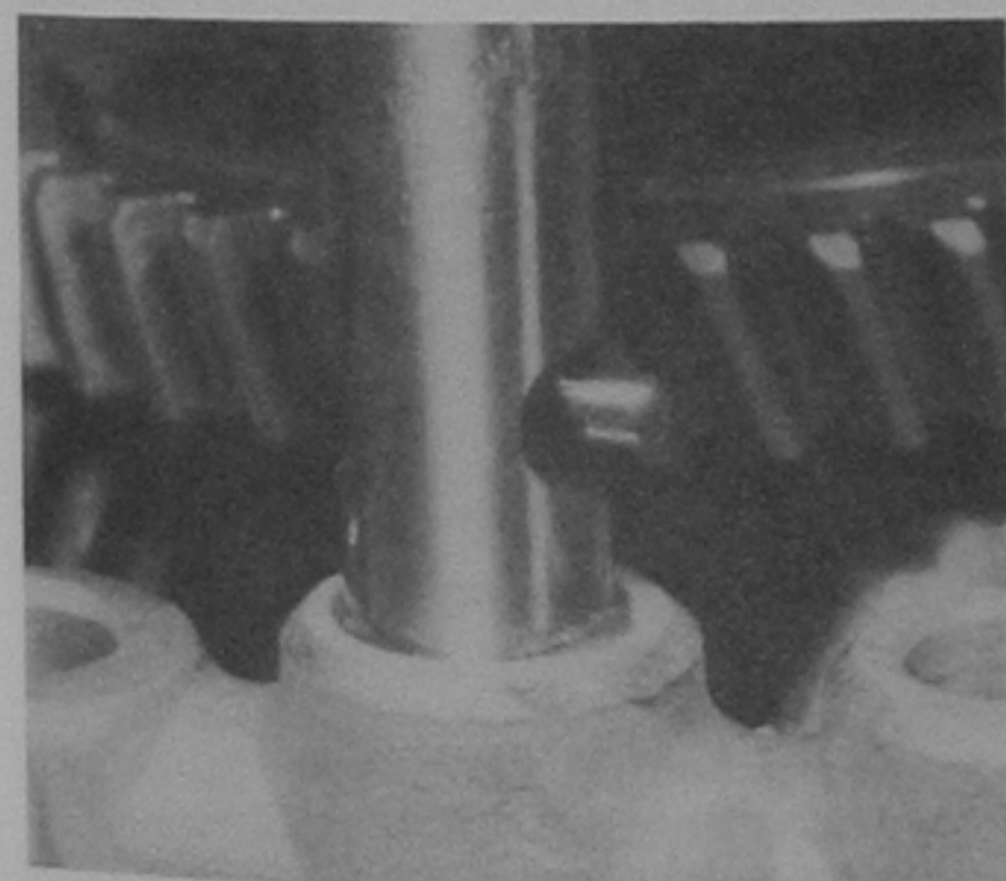
9.8 Interlock plunger in 3rd/4th selector shaft
