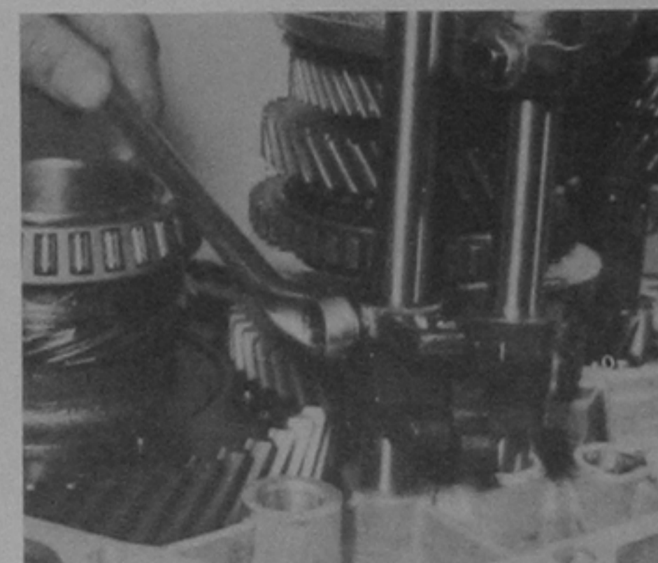
9.9B Tightening 1st/2nd selector fork lockbolt
