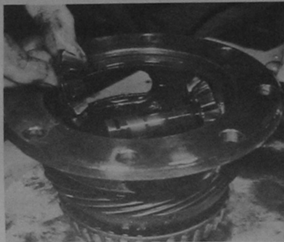
8.2D Removing differential planet gears
