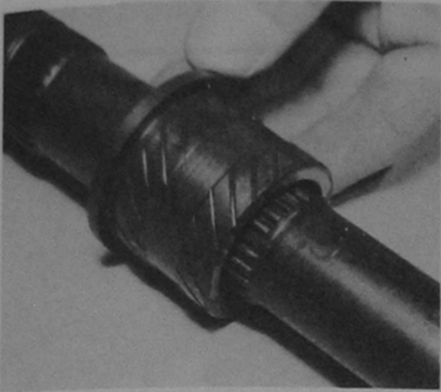
7.6 1st speed gear bush on mainshaft
